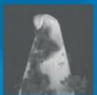
Electron micrograph images of 27G needles (1000x magnification) after injection into mice demonstrating the potential for dulling of the needle and contamination when reused.
