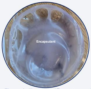
**Figure 6:** illustrates different types of EOL PV panel waste delaminated by using different kind encapsulated available at the time when they manufactured.
