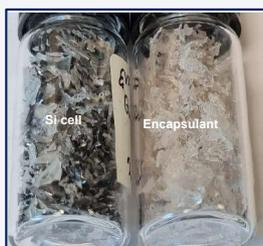
**Figure 5:** Extraction of EVA from toluene by evaporation filtration and manually recovered fractions of PV cell for further elemental analysis.
