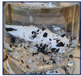
**Figure 3:** Chemical treatment of EOL PV panel waste sample by the dissolution process in an organic solvent basically toluene.
