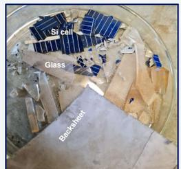
**Figure 4:** Laminated PV panel layered structure separated into different components after immersing into toluene.
