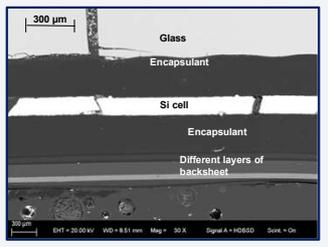
**Figure 2:** Electron microscopy cross section image of end-of-life c-Si solar panel showing composition and different layers present in solar cell. Chemical composition can be determined by EDX measurements.
