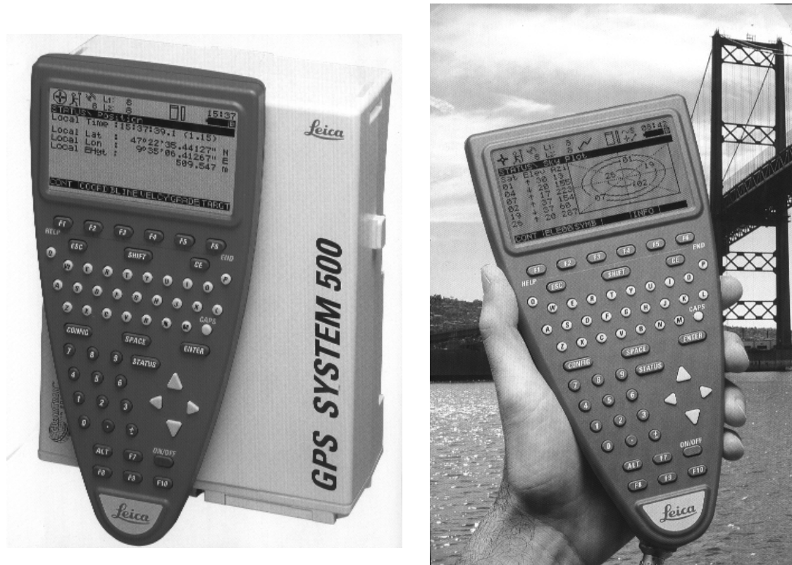
Figure 23: Two Examples of Read-out from a GPS Receiver: satellites available for observation in the sky (left) and the computed latitude, longitude and elevation (right) (Courtesy of Leica Corp).
