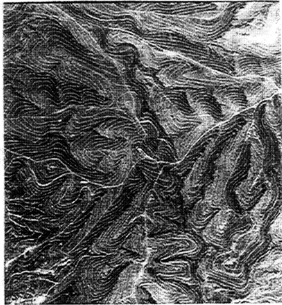
Figure 2: An Image, Stereoscopically Observed, with Contour Lines Superimposed and a 1:50,000 Map of the Same Area
